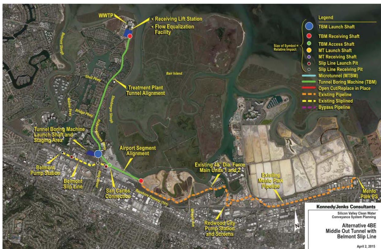
Figure 1-2. Schematic diagram of the proposed project
