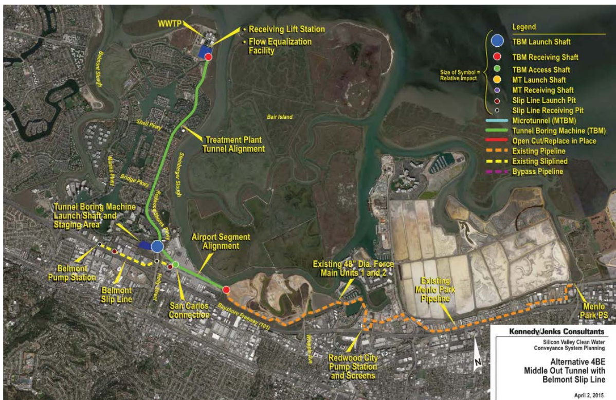
Figure 2-7. Schematic diagram of the proposed Conveyance System Project
