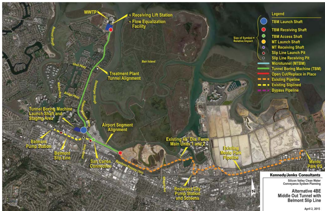
Figure 1-2. Schematic diagram of the proposed project
