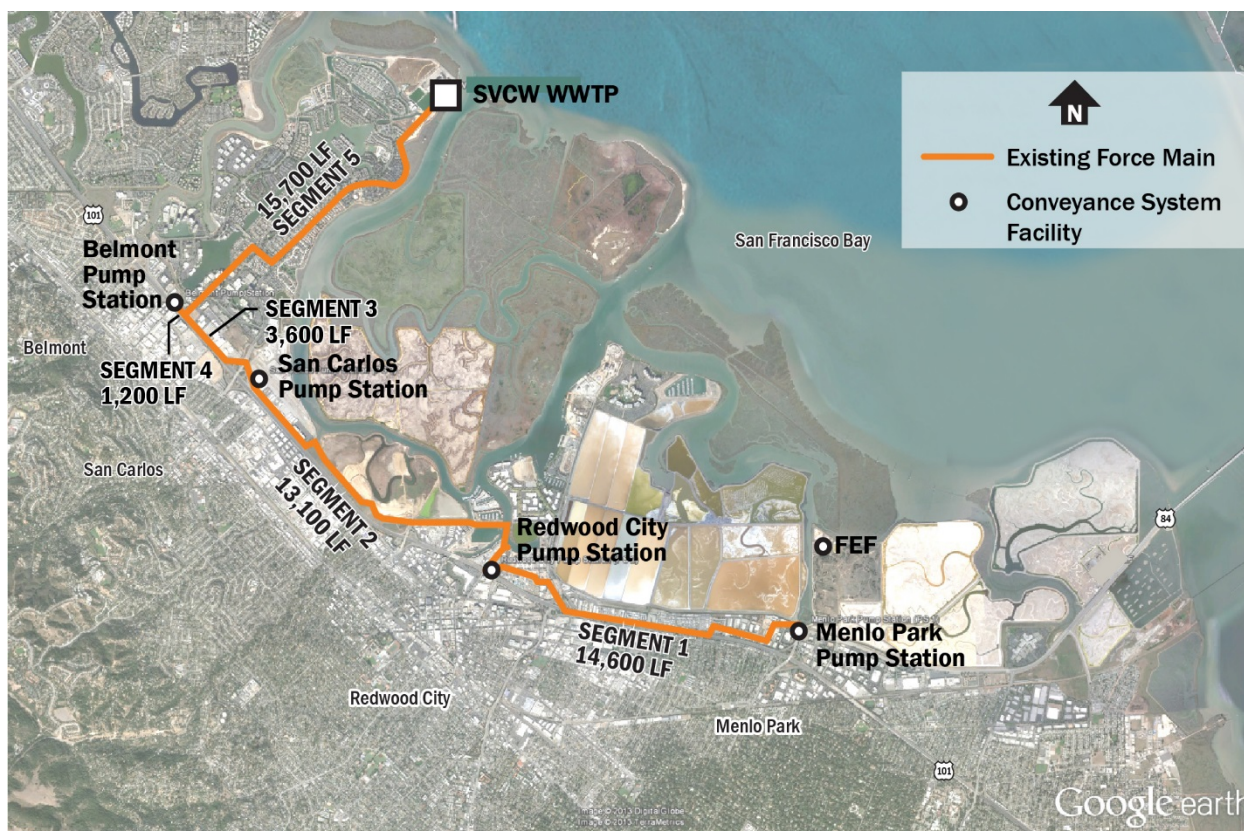
Figure 2-4. SVCW existing conveyance system
