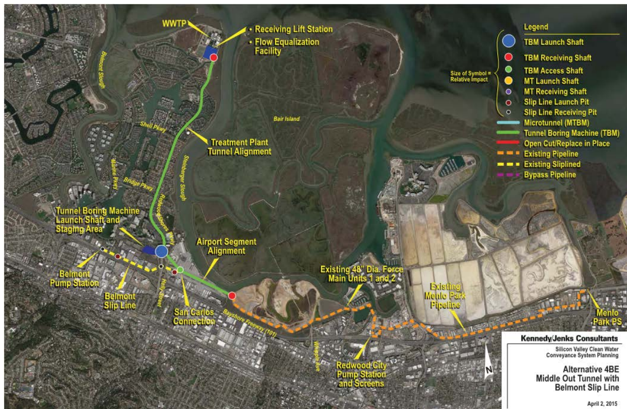
Figure ES-1. Schematic diagram of the proposed Conveyance System Project
