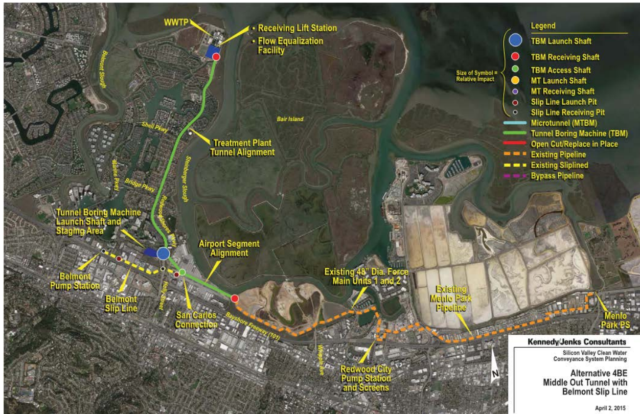
Figure ES-1. Schematic Diagram of Alternative 4BE (Source: Kennedy/Jenks Consultants)
