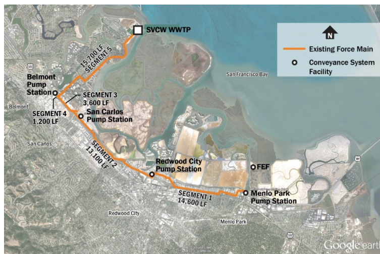
Figure 1-1. SVCW Existing Conveyance System
