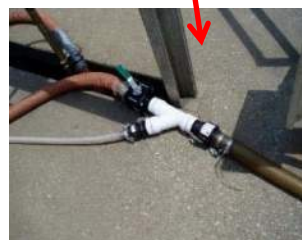
Splitter – Used to maintain overflow rate in settler
