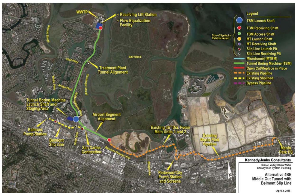
Figure 1-2. Schematic diagram of the proposed project (Source: Kennedy/Jenks Consultants)
