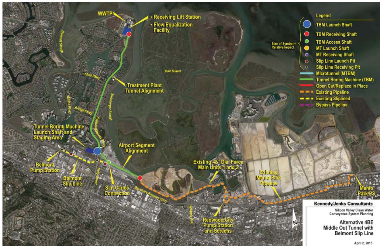
Figure ES-1. Schematic diagram of proposed Conveyance System Project
